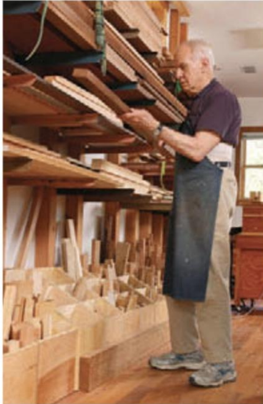
Lumber storage. Houck's wall-mounted lumber rack uses space efficiently because the angle-iron requires no bracing. A graduated set of boxes underneath keeps scrap
